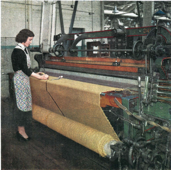
This loom is the first of two looms used in the manufacture of Chenille Axminster carpets.
