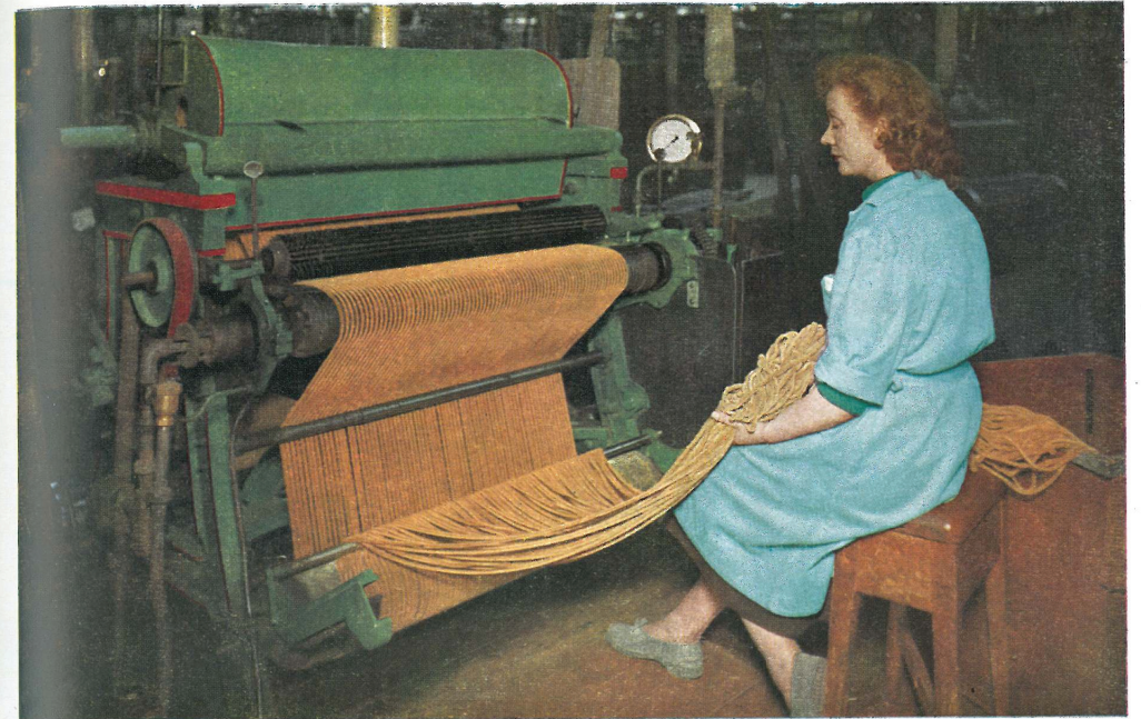
The chenille is now cut into strips on the fur-cutting machine, to make it ready for the carpet-weaving process.
