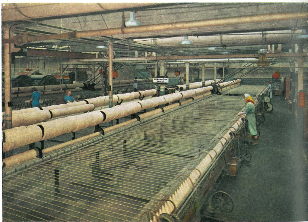
Spinning mules at our Brookside Street mill working on "Blend 17"—the Coronation Yarn.
